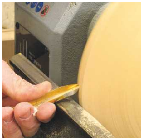
▲ Pic.5 A tool sharpened like this is so versatile: a push technique on the edge gives the best finish; a pull cut could lead to the tool catching, especially if it overhangs the toolrest too much
